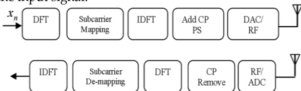
Fig. 6 Transmitter and receiver structure of SC-FDMA
